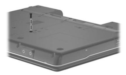
Where used: 1 screw that secures the optical drive to the computer
